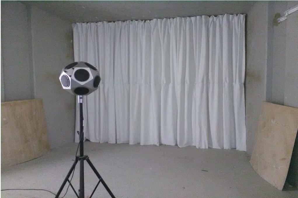
**Figura 2\_ Reverberation chamber with Sample Configuration 1**
